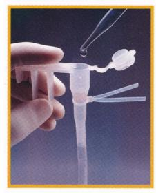
Cellu • Sep Filler Funnels make loading and unloading dialysis tubing easy: Cut membrane tube to length and clamp at one end, slip the open end onto the polypropylene funnel and secure with the rubber loop fastener. Open snap cap, fill with sample, and hang in container. Funnels are supported by a three-notched universal hanger that fits over the edge of common vessels.
