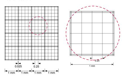
The depth of the Fuchs-Rosenthal counting chamber is 0.2 mm. In total the grid covers 16 mm² and contains 16 large squares of each 1 mm length of the edge. These large squares are separated by triple lines with a space of 0.01 mm between each other. The distance between the center lines is 1 mm. All 16 large squares are subdivided into 16 small squares of a side length of 0.25 mm.
