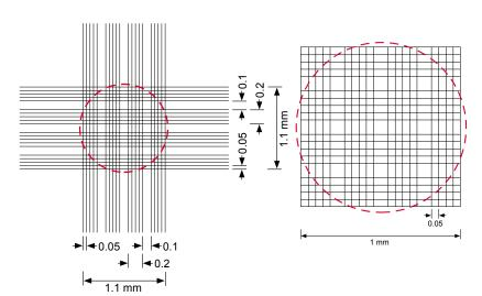
The depth of the Thoma new counting chamber is 0.1 mm. The grid covers an area of 1.1 x 1.1 mm $^2$ . It is subdivided in 16 group squares with a side length of 0.2 mm.
