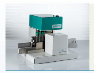
The VACUETTE® UNICAP Rack Decapper can decap all VACUETTE® tube dimensions directly in analyser racks which are already in use in the laboratory.
