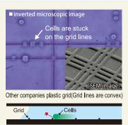
Easier to count because cells do not get stuck on the grid lines that are molded in the groove form. Cells are easier to be
