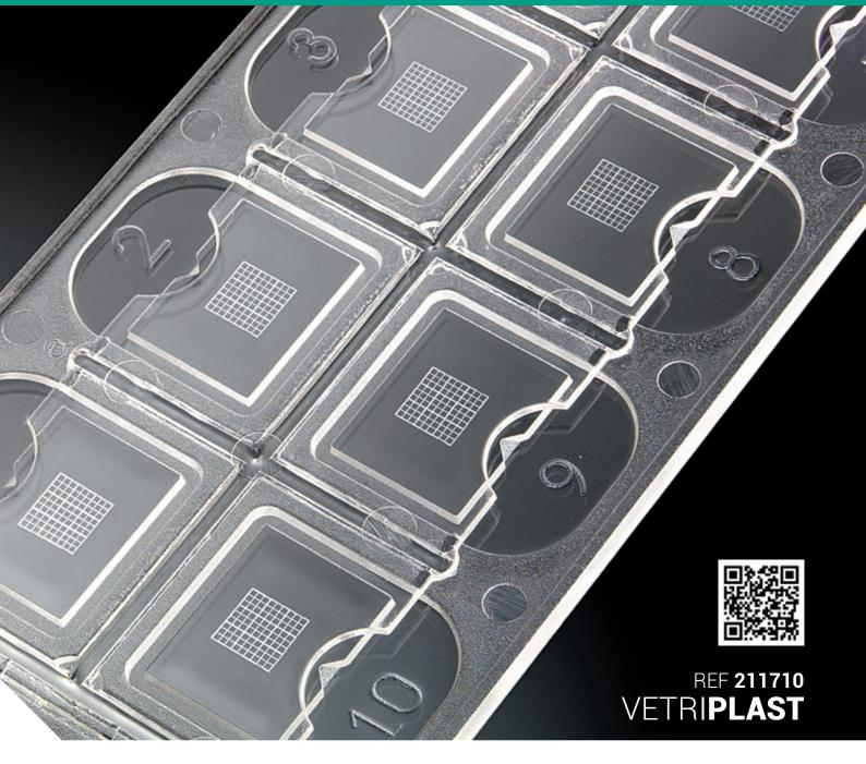
In the **Pentasquare** slide with counting grid, the microscopic counting of the cells present in the urine sediment, is based on the same principle of the glass counting chambers actually present on the market (Bürker, Thoma-Zeiss, Neubauer).
