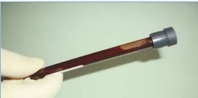
Fig. 27: Air bubble as indicator for mixing
